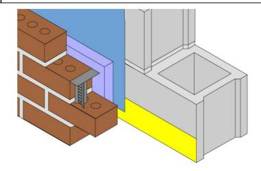
WIRELOCK Plastic Louvered Weep Vent allows air to pass through freely and water to weep out while inhibiting reverse passage of water.
