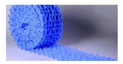
WIRELOCK Mortar Stop helps prevent mortar droppings from clogging the weep vents, thus allowing for increased moisture drainage and air movement within the wall.
