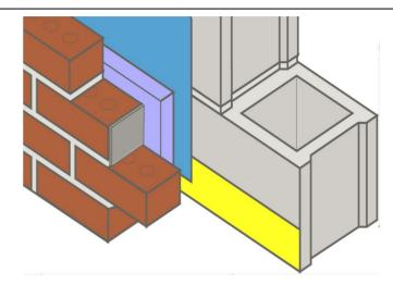
WIRELOCK Cell Vents, with a honeycomb design, ensures that moisture can migrate out of the cavity, air can circulate into the cavity and insects and other debris cannot enter through the weep holes.
