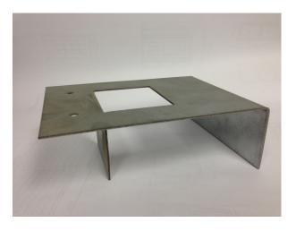
WireLock Partition Top Anchors provide lateral shear resistance at the upper limit of masonry walls, they permit vertical deflection of the slab above, without transferring compressive loads to the masonry wall below.
