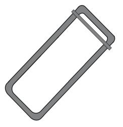
WIRELOCK Rectangular Anchor with Restraint Bar is used in conjunction with Box Ties for tying brick veneer to block.
