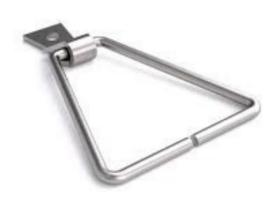
WIRELOCK Dovetail Tri-Ties are a flexible tie used to anchor masonry to concrete. The dovetail fits into a slot attached inside the concrete backup. The hole in the middle of the dovetail also allows the tie to be screwed into the concrete backup if a slot is not being used.
